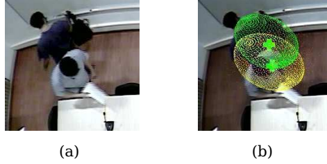
Figure 4.6: Particles from the tracker A (yellow ellipsoid) falling into the exclusion zone of tracker B (green ellipsoid) will be penalized by a multiplicative factor \alpha \in [0, 1] .
