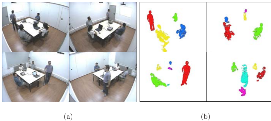
Fig. 1. In (a) there is an example frame from a multiview camera environment: Smart-Room at UPC. In (b) the result of a foreground segmentation and extraction of labeled blobs
